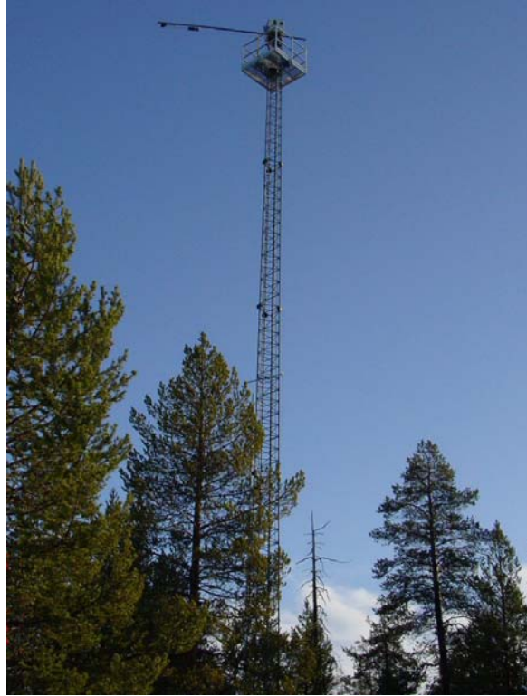
Fig. 1.4. The spectrometer installed into the 30-m-high mast. The measurement head is located on the top in a boom 3.80 meter distance from the mast. The boom is rotated by turning the pole during a measurement in order to measure a forested target area and a forest opening. As a result forest and open area VIS/IR reflectance spectra are obtained. The spectrometer is installed into a weather resistant cover box. The measurement head has a 25 degrees field-of-view, and it is directed 11^\circ off the nadir. A large-view control/reference image acquisition camera is also included into the system. A special moving white reference panel provides on-site calibration. Reference measurements within the mast area include continuous automatic observations ground surface temperature and soil moisture, snow depth and snow water equivalent (SWE).
