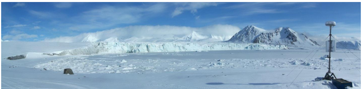
Figure. 22. Ice Cliff of Hansbreen and front position monitoring station with laser distance ranger and panoramic radar. Riegl laser distance meter is giving high time resolution (every 10 min) and high accuracy ( \pm 0.5 m) point data (weather depended record). Garmin panoramic radar provides data on entire cliff position every day during day and night and bad weather, with low accuracy ( \pm 12.5 m). Photo by M. Laska
